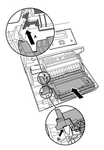
Push the automatic duplex unit down (1) (and paste the label (2) provided with DP-CL18 only so it is overlapped on the jam clear label that has been pasted).
